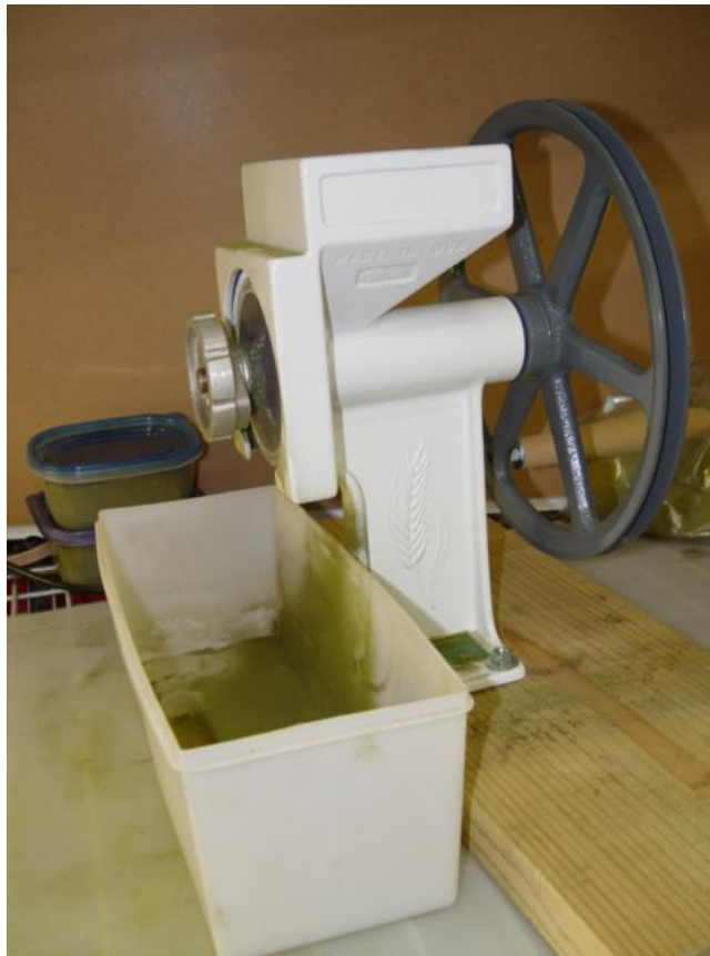
Figure 14. Photograph of the mill used to pulverize dried algae.
