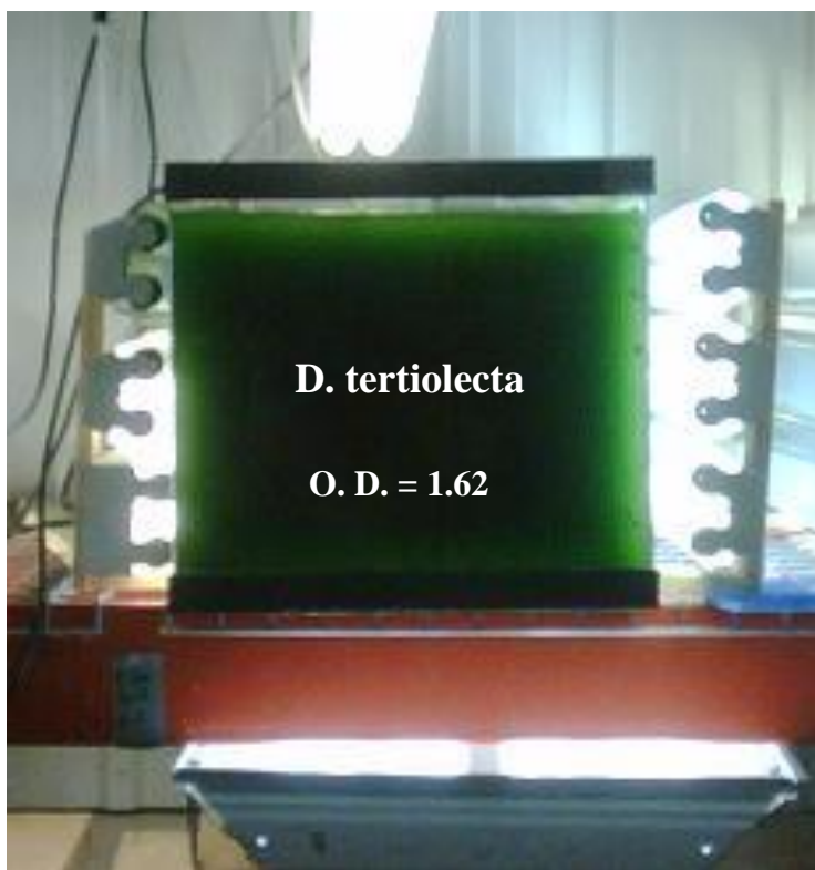
Figure 10. Picture showing the light penetration into a D. tertiolecta culture with an OD=1.62.
