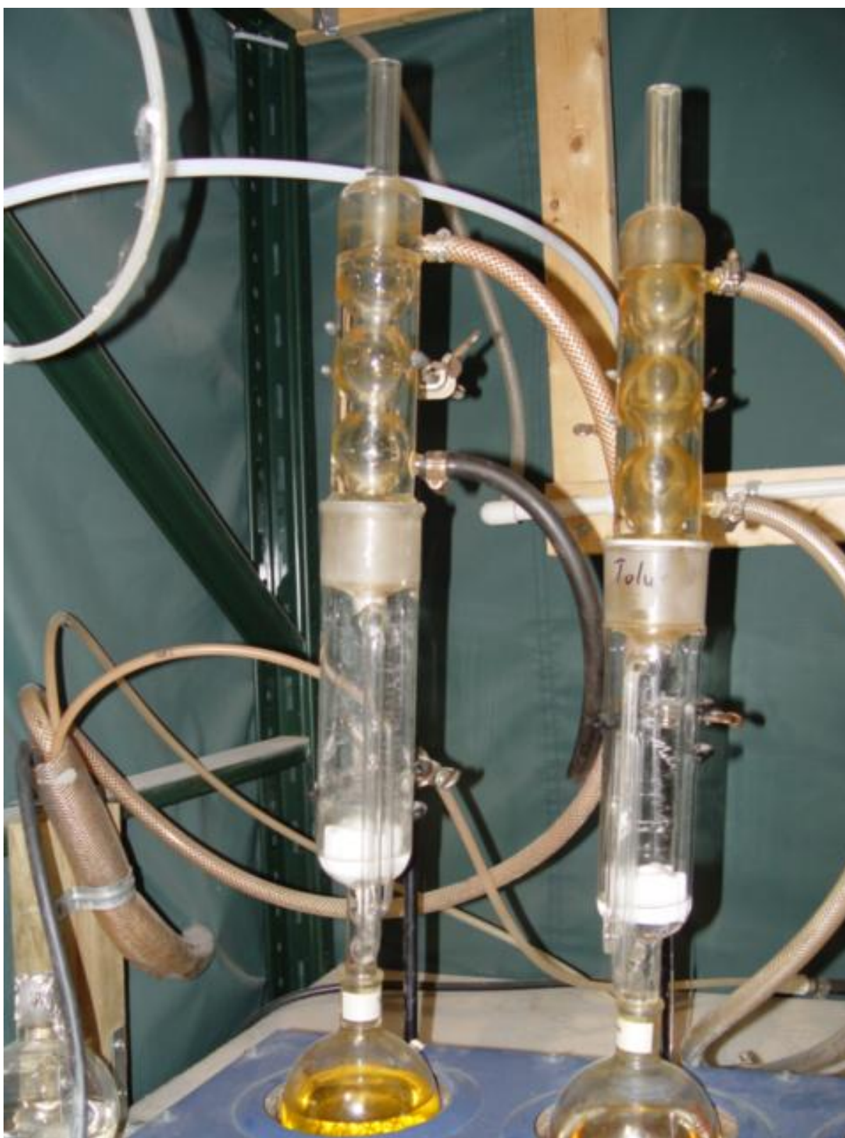
Figure 18. Soxhlet apparatus for extracting lipids from algae.
