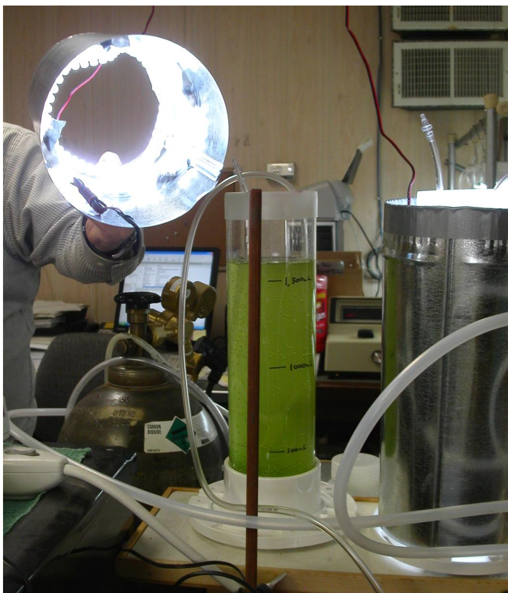
Figure 3. Photo bioreactor (PBR) showing LED light source in a spiral pattern on the internal side of the tubular photo shield.
