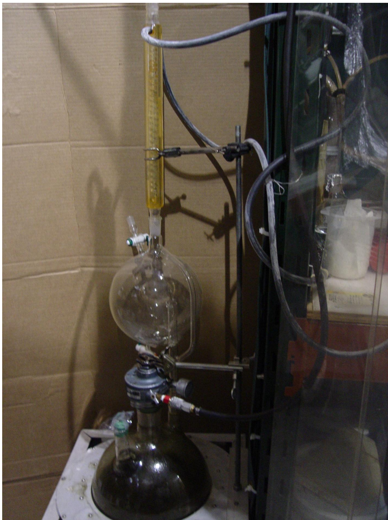
Figure 17. Reflux apparatus containing algae & solvent, with stirring and heat.
